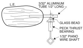
PROP BLADES ARE 1/32" SHEET FORMED ON A 3" CYLINDER. SET EACH BLADE WITH THE LEADING EDGE 15 DEGREES LEFT FROM VERTICAL ON THE CYLINDER. MAKE 4 IDENTICAL BLADES FOR 2 PROP ASSEMBLIES. PROP SPARS ARE MADE FROM BAMBOO ROUNDED TO 1/16" DIAMETER. A GOOD SOURCE FOR BAMBOO IS SHISH KABOB SKEWERS. GLUE THE SPARS INTO THE ALUMINUM TUBE. USE REGULAR MODEL AIRPLANE CEMENT FOR THIS SO PITCH ADJUSTMENTS CAN BE MADE BY SOFTENING THE GLUE WITH ACETONE.
