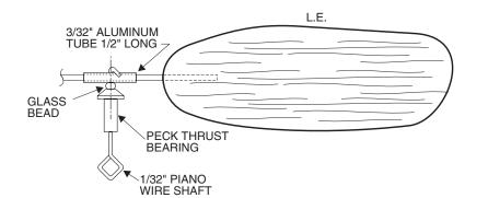
PROP BLADES ARE 1/32" SHEET FORMED ON A 3" CYLINDER. SET EACH BLADE WITH THE LEADING EDGE 15 DEGREES LEFT FROM VERTICAL ON THE CYLINDER. MAKE 2 IDENTICAL BLADES FOR THE PROP ASSEMBLY. PROP SPARS ARE MADE FROM BAMBOO ROUNDED TO 1/16" DIAMETER. A GOOD SOURCE FOR BAMBOO IS SHISH KABOB SKEWERS. GLUE THE SPARS INTO THE ALUMINUM TUBE. USE REGULAR MODEL AIRPLANE CEMENT FOR THIS SO PITCH ADJUSTMENTS CAN BE MADE BY SOFTENING THE GLUE WITH ACETONE.
