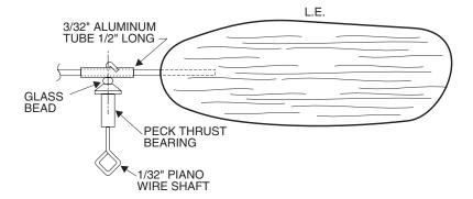
PROP BLADES ARE 1/32" SHEET FORMED ON A 3" CYLINDER. SET EACH BLADE WITH THE LEADING EDGE 15 DEGREES LEFT FROM VERTICAL ON THE CYLINDER. MAKE 2 IDENTICAL BLADES FOR THE PROP ASSEMBLY. PROP SPARS ARE MADE FROM BAMBOO ROUNDED TO 1/16" DIAMETER. A GOOD SOURCE FOR BAMBOO IS SHISH KABOB SKEWERS. GLUE THE SPARS INTO THE ALUMINUM TUBE. USE REGULAR MODEL AIRPLANE CEMENT FOR THIS SO PITCH ADJUSTMENTS CAN BE MADE BY SOFTENING THE GLUE WITH ACETONE.
