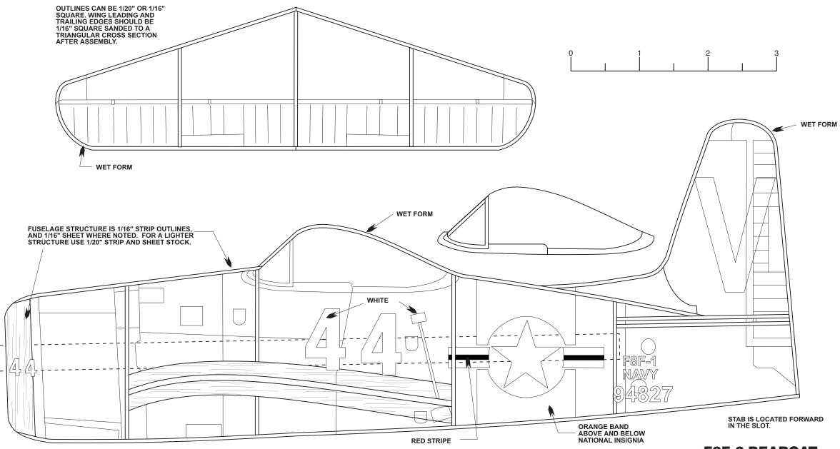
IF A PLASTIC PROP IS USED, USE A 6" PROP, OR A 7" PROP CUT TO 6". SHAVE TO LIGHTEN.
