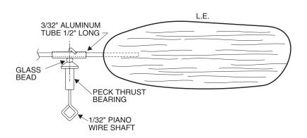
PROP BLADES ARE 1/32" SHEET FORMED ON A 3" CYLINDER. SET EACH BLADE WITH THE LEADING EDGE 15 DEGREES LEFT FROM VERTICAL ON THE CYLINDER. MAKE 2 IDENTICAL BLADES FOR THE PROP ASSEMBLY. PROP SPARS ARE MADE FROM BAMBOO ROUNDED TO 1/16" DIAMETER. A GOOD SOURCE FOR BAMBOO IS SHISH KABOB SKEWERS. GLUE THE SPARS INTO THE ALUMINUM TUBE. USE REGULAR MODEL AIRPLANE CEMENT FOR THIS SO PITCH ADJUSTMENTS CAN BE MADE BY SOFTENING THE GLUE WITH ACETONE.
