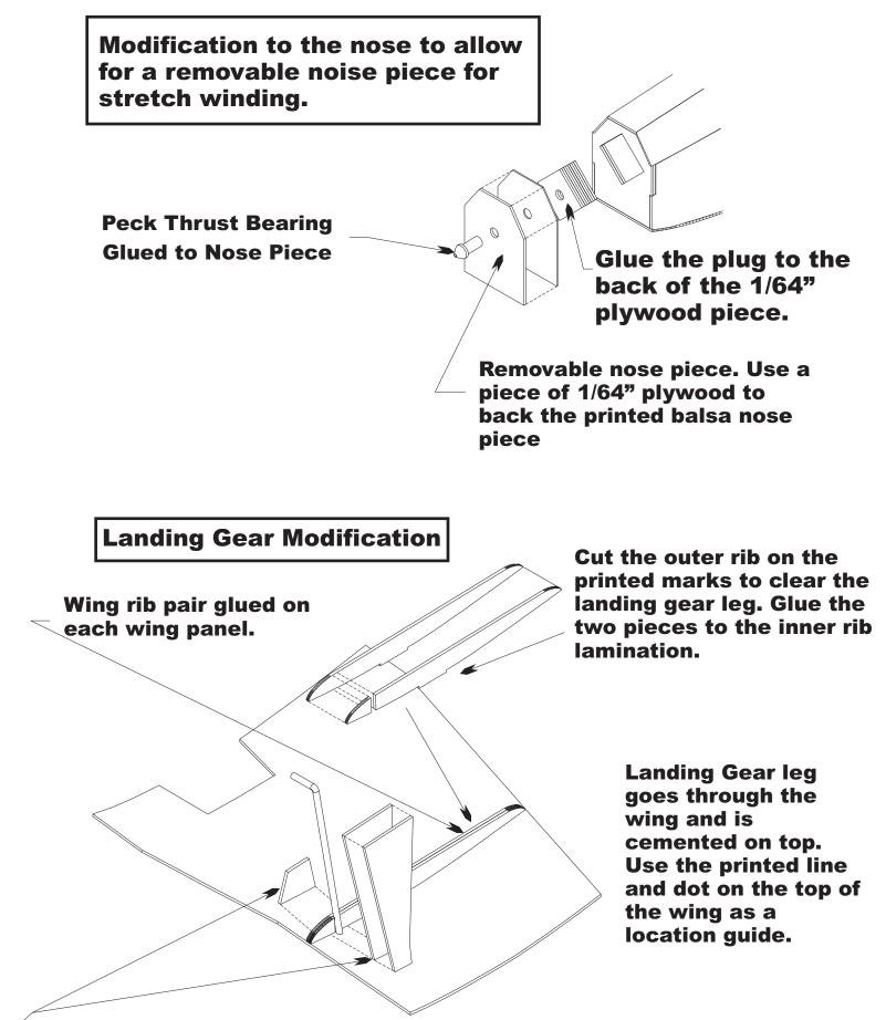
These pieces sandwich the gear leg piano wire. The gear cover is a two piece lamination glued to the rib and the gear leg.
